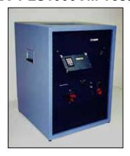
The PLS1000CM automatic tester is designed primarily to do SURGE testing either as single pulses or with Forward and Reverse bias, according to methods 4066-1 or 4066-2. In addition, it can also test VF with rectangular pulses and THERMAL RESPONSE either in DVF (mV) or degrees per watt.
