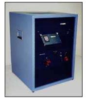
The PLS500 automatic tester is designed primarily to do SURGE testing either as single pulses or with Forward and Reverse bias, according to methods 4066-1 or 4066-2. In addition, it can also test VF with rectangular pulses and THERMAL RESPONSE either in DVF (mV) or degrees per watt. All three test types may be performed in a single test program.
