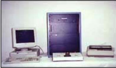
The FEC200 is an automatic computer controlled diode and rectifier tester. It is controlled by a standard PC-compatible computer running FreeDOS. The testing software is very powerful, yet the easiest to use.
